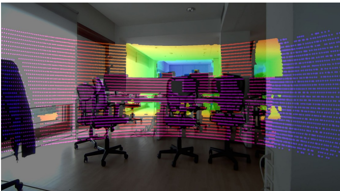
Figure 7. Point cloud reprojection onto RGB image, after intrinsic and extrinsic calibration.
