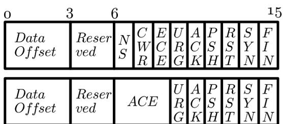
Figure 4. Bytes 13 and 14 of TCP header
