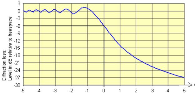
Figure 7. Diffraction loss of a “knife-edge” versus parameter  $v$  [7]
