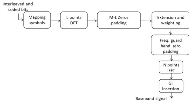
Figure 6. SC-FDMA transceiver architecture enabling frequency holes.
