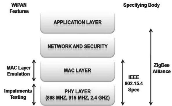
Figure 21. ZIGBEE stack [22].
