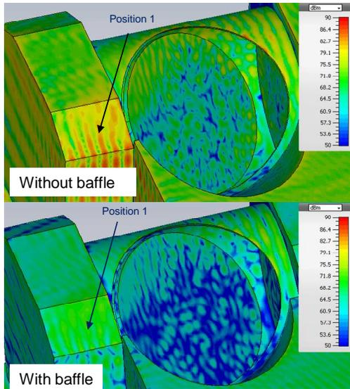
Figure 12. Simulated field strength at MWS assuming real antenna pattern;  $f=8.2$  GHz
