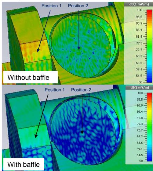
Figure 10. Simulated field strength at MWS assuming radiating dipole;  $f=8.2$  GHz
