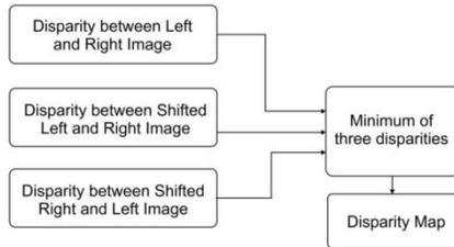
Figure 13. Process of disparity estimation.
