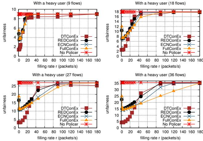
Figure 18. Unfairness with DTConEx, REDConEx, ECNConEx and FullConEx
