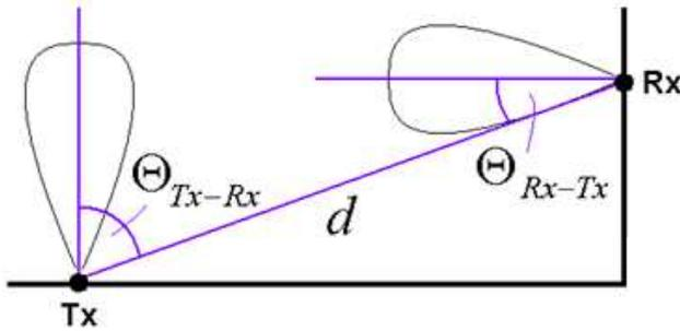
Figure 3. General definition of angles between transmitter and receiver
