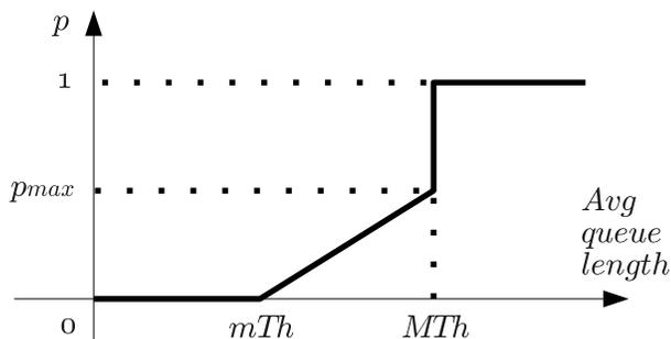
Figure 2. Random Early Detection dropping/ marking function
