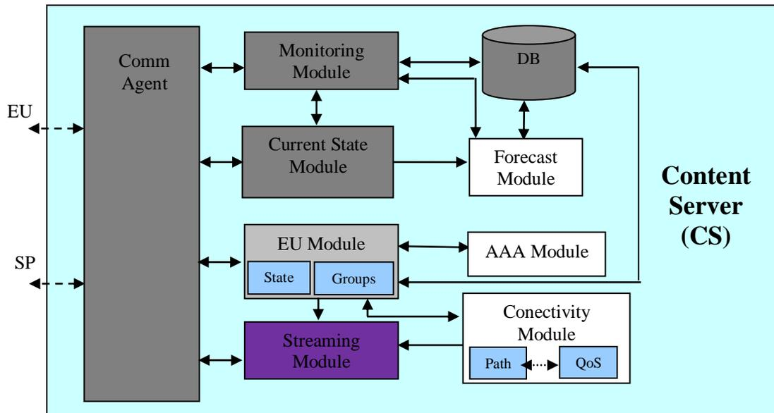
Figure 4. The Content Server software architecture
