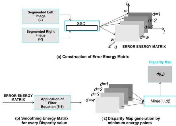
Figure 15. Method using global error energy minimization by smoothing functions.
