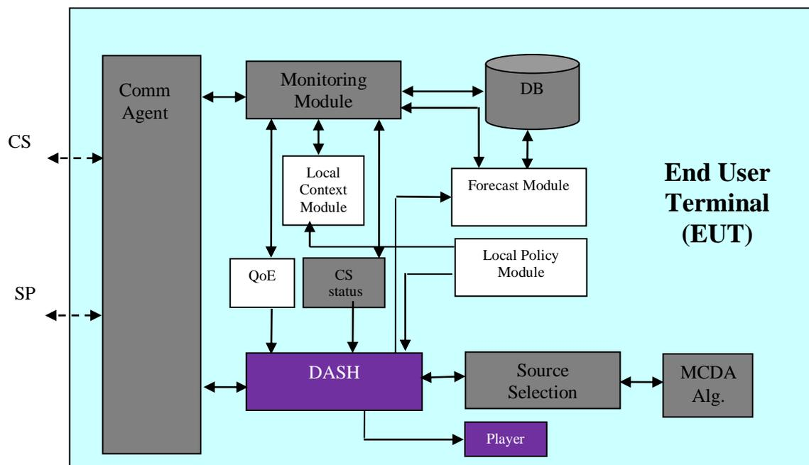
Figure 3. The End User Terminal software architecture
