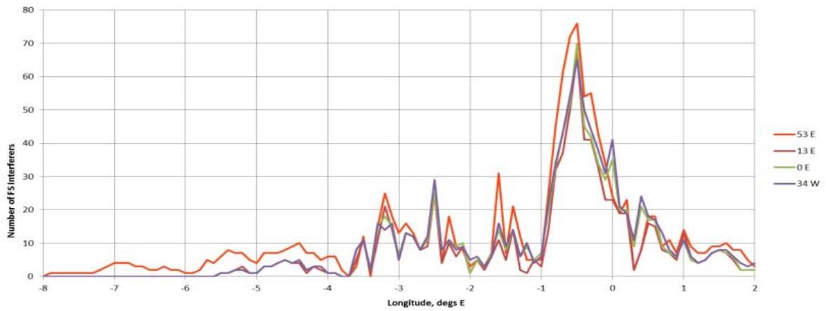
Figure 13. Number of FS interferers for different satellite locations (longitude)
