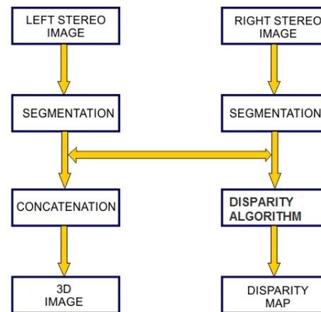
Figure 4. Segmentation based stereo matching system.
