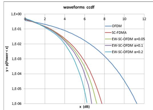
Figure 5. Complementary Cumulated Density Function of waveforms instantaneous power. 512 sub-carriers are used for simulations.
