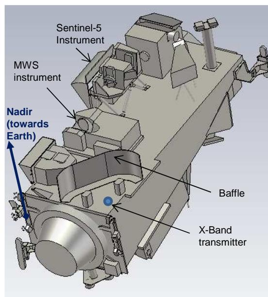
Figure 2. Model of “Satellite A” being part of MetOp Second Generation: Exemplary transmitter and instrument receiver positions
