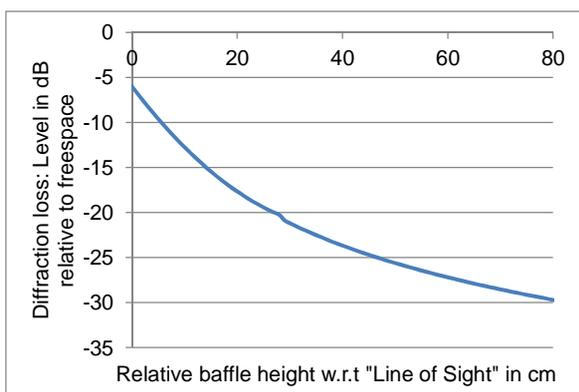
Figure 8. Diffraction loss of a “knife-edge” versus  $h$  assuming  $d_1 = 1.5$  m,  $d_2 = 1.5$  m and  $f = 8.2$  GHz
