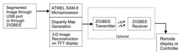
Figure 2. Hardware implementation of stereo matching .
