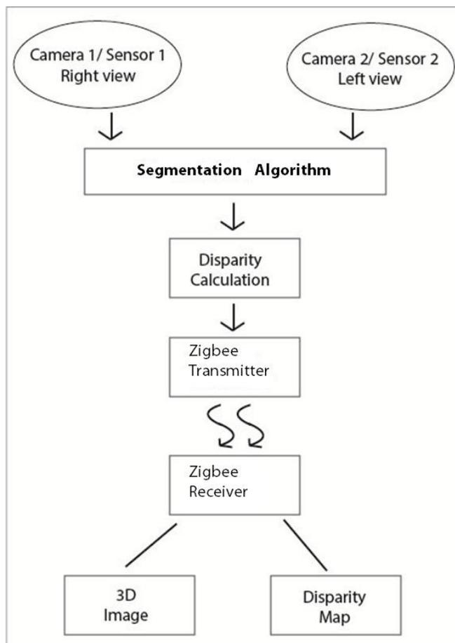
Figure 25. Steps in wireless transmission of stereo images and its disparity levels.
