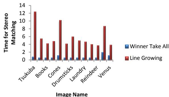
Figure 27. Time required for stereo matching in seconds using LG and WTA.
