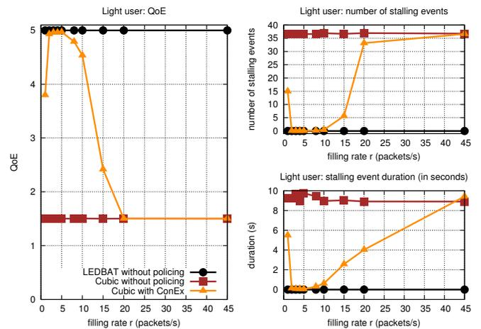
Figure 22. QoE of light users, the number of stalling events and the duration of a single stalling event
