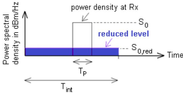
Figure 4. Temporal effects on power spectral density
