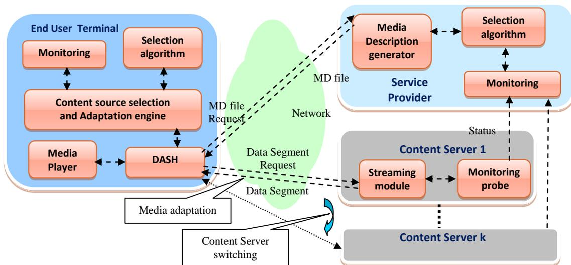
Figure 1. DISEDAN general architecture; DASH - Dynamic Adaptive Streaming over HTTP
