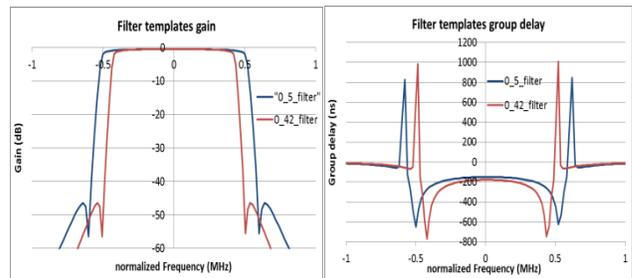
Figure 17. IMUX filter templates models : 0\_42\_filter and 0\_5\_filter.
