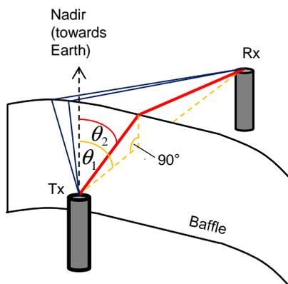
Figure 13. Principal scenario involving diffracted paths
