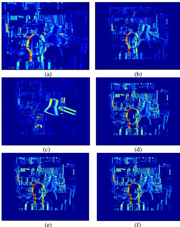
Figure 14. Disparity map using WTA and various segmentation techniques (a) Original (b) Mean shift (c) K-means (d) PSO (e) DPSO (f) FO-DPSO.
