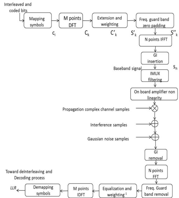
Figure 3. SC-FDMA transceiver architecture.
