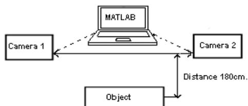
Figure 1. Block diagram of camera setup.
