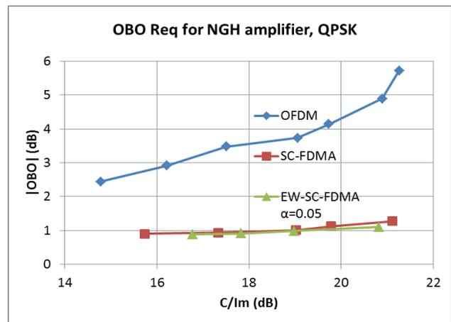
Figure 13. Comparison of waveforms in terms of OBO vs  $C/I_m$  when no frequency holes are inserted and without interference, for NGH amplifier.
