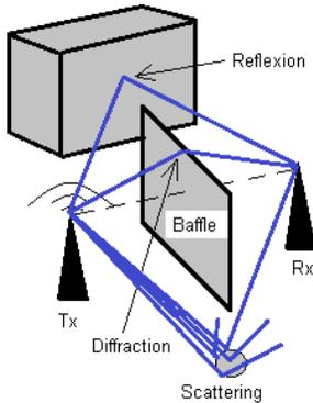
Figure 5. Multipath propagation
