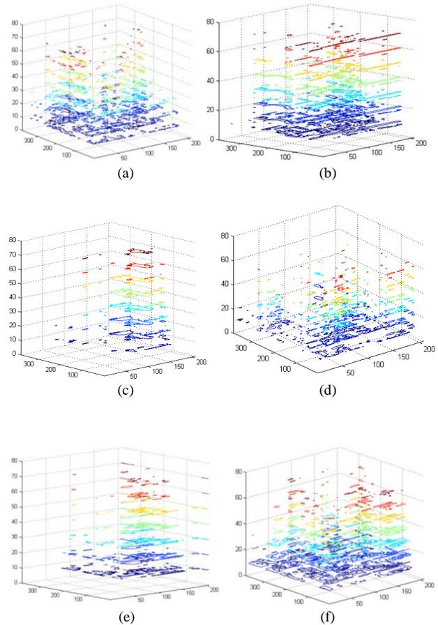
Figure 19. Depth Map using various segmentation techniques and LG for Tsukuba (a) Original (b) Mean Shift (c) K-means (d) PSO (e) DPSO (f) FO-DPSO.
