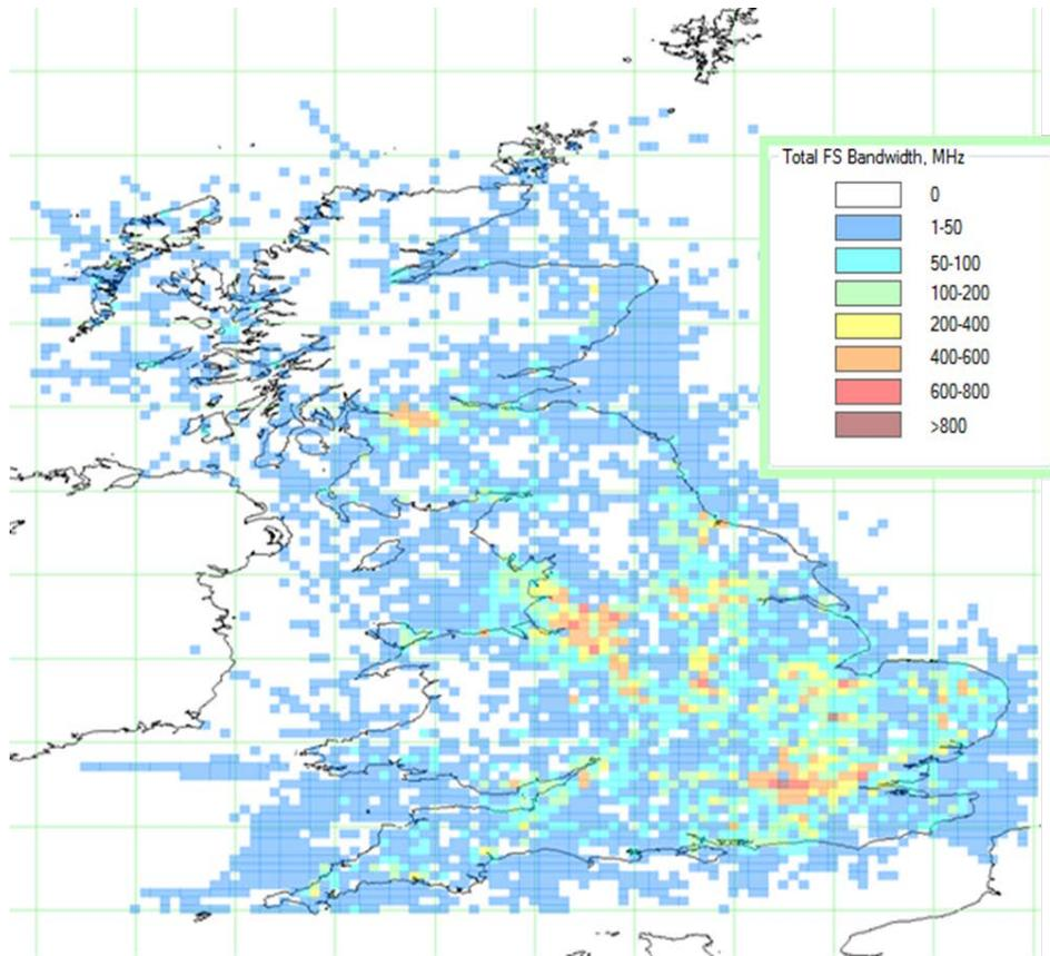
Figure 10. Interfering spectrum at -154 dBW/MHz for the UK
