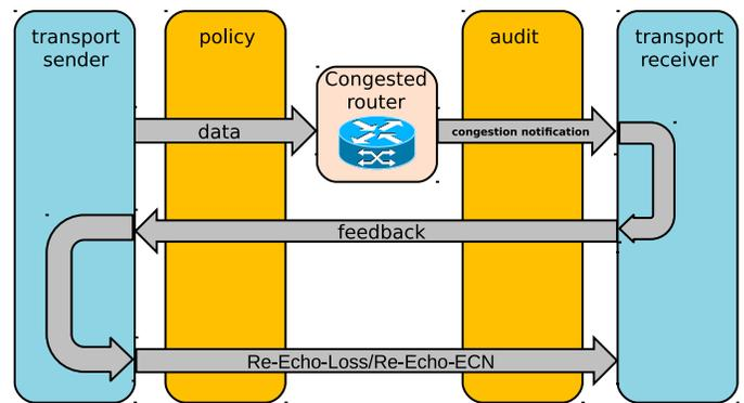
Figure 1. ConEx mechanism
