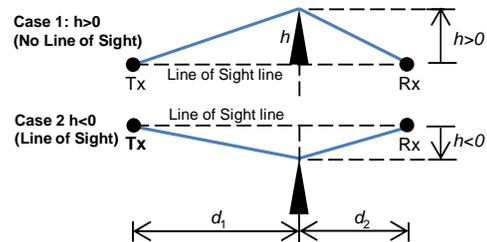
Figure 6. Diffraction at a “knife-edge” for two cases: “No Line of Sight” and “Line of Sight”
