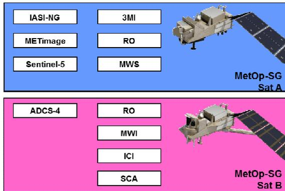
Figure 1. Allocation of payload instrument on-board the MetOp-SG satellites; left: Customer Furnished Instruments; right: Contractor Furnished Instruments
