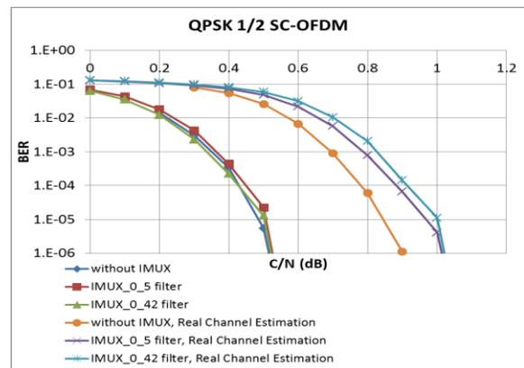
Figure 18. IMUX filter effect over SC-FDMA performances.
