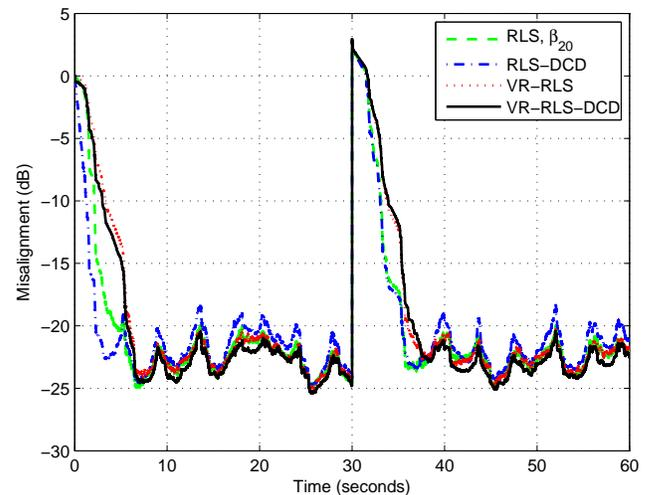
Figure 6. Misalignment of the regularized RLS (using  $\beta_{20}$ ), RLS-DCD, VR-RLS, and VR-RLS-DCD algorithms. The input signal is speech,  $L = 512$ , and ENR = 20 dB. Echo path changes at time 30 seconds.
