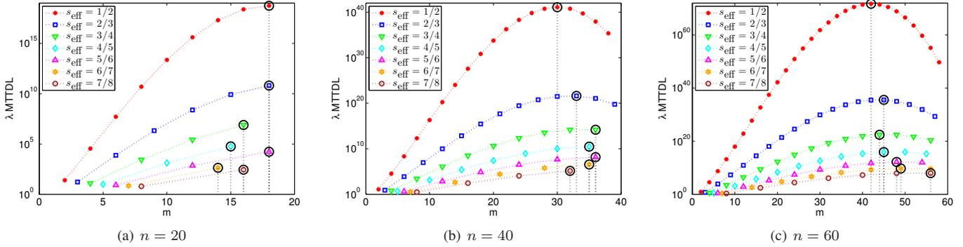
Figure 19. Normalized  $\text{MTTDL}^{\text{declus}}$  vs. codeword length for  $s_{\text{eff}} = 1/2, 2/3, 3/4, 4/5, 5/6, 6/7,$  and  $7/8$ ;  $\lambda/\mu = 0.001$  and exponential rebuild times.
