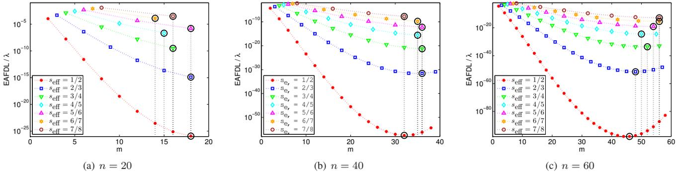
Figure 9. Normalized  $\text{EAFDL}^{\text{declus}}$  vs. codeword length for  $s_{\text{eff}} = 1/2, 2/3, 3/4, 4/5, 5/6, 6/7,$  and  $7/8$ ;  $\lambda/\mu = 0.001$  and deterministic rebuild times.
