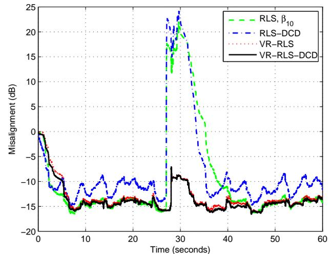
Figure 9. Misalignment of the regularized RLS (using  $\beta_{10}$ ), RLS-DCD, VR-RLS, and VR-RLS-DCD algorithms. The input signal is speech,  $L = 512$ , and ENR = 10 dB. Near-end speech appears between time 27 and 30 seconds (double-talk scenario).
