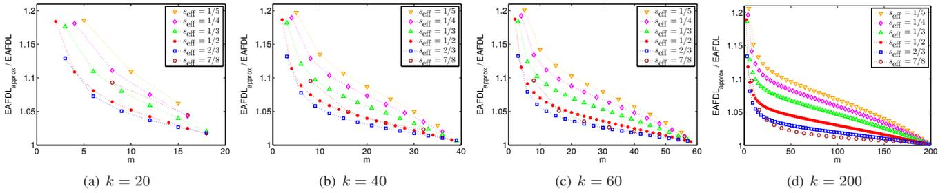
Figure 6.  $\text{EAFDL}_{\text{approx}}^{\text{sym}} / \text{EAFDL}^{\text{sym}}$  ratio vs. codeword length for  $s_{\text{eff}} = 1/5, 1/4, 1/3, 1/2, 2/3,$  and  $7/8$ .
