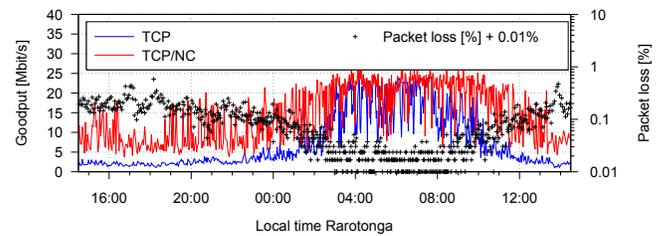
Figure 9. Goodput of uncoded (blue) and coded (red) TCP transfers between Auckland (New Zealand) and Rarotonga (Cook Islands) via a real MEO satellite link. Note that the goodput is quite comparable during the low demand hours (late night and early morning) with low packet loss from queue oscillation. During peak times, coded goodput significantly exceeds uncoded goodput. Peak link utilisation on this link was around 50%.
