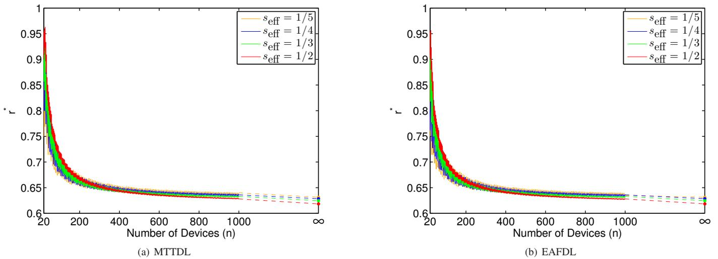
Figure 14.  $r^*$  vs. number of devices  $n \rightarrow \infty$ ,  $s_{\text{eff}} = 1/5, 1/4, 1/3,$  and  $1/2$ ;  $\lambda/\mu = 0.001$  and deterministic rebuild times.
