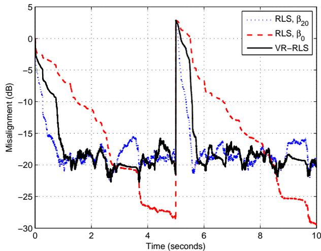
Figure 4. Misalignment of the regularized RLS algorithm (using different constant values of the regularization parameter) and the VR-RLS algorithm. The input signal is speech,  $L = 128$ , and ENR = 20 dB. Echo path changes at time 5 seconds.
