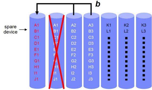
Figure 3. Rebuild under clustered placement.
