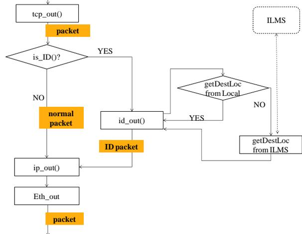
Figure 6. Packet encapsulation process.
