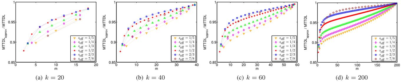
Figure 5.  $\text{MTTDL}_{\text{approx}}^{\text{sym}} / \text{MTTDL}^{\text{sym}}$  ratio vs. codeword length for  $s_{\text{eff}} = 1/5, 1/4, 1/3, 1/2, 2/3,$  and  $7/8$ .
