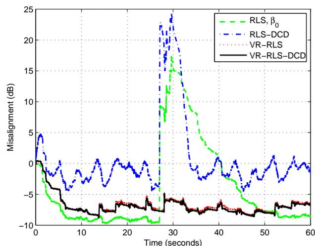
Figure 11. Misalignment of the regularized RLS (using  $\beta_0$ ), RLS-DCD, VR-RLS, and VR-RLS-DCD algorithms. The input signal is speech,  $L = 512$ , and ENR = 0 dB. Near-end speech appears between time 27 and 30 seconds (double-talk scenario).
