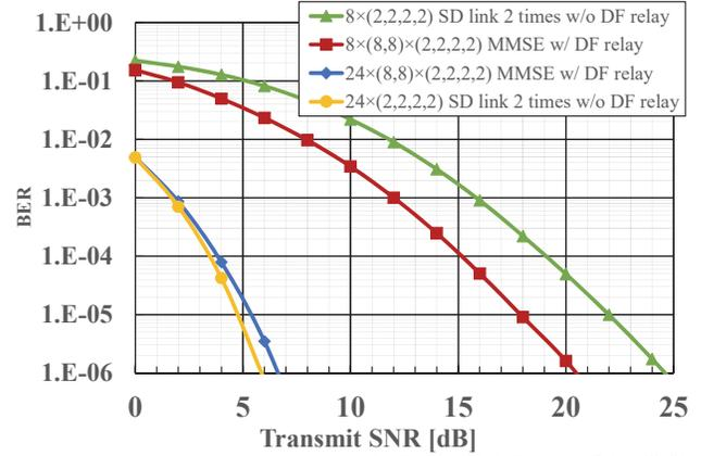
Figure 11. BER characteristics of  $8 \times (8,8) \times (2,2,2,2)$  or  $24 \times (8,8) \times (2,2,2,2)$  model (Transmission rate to each user is 6 (bps/Hz) and 64QAM, 16QAM or QPSK is optimally selected to minimize the BER.)
