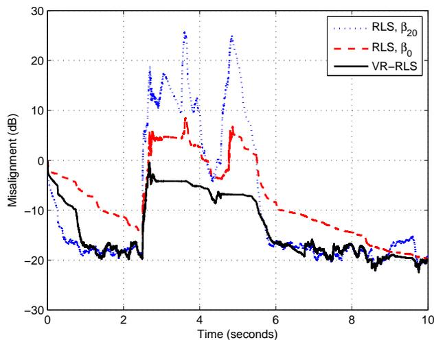
Figure 5. Misalignment of the regularized RLS algorithm (using different constant values of the regularization parameter) and the VR-RLS algorithm. The input signal is speech,  $L = 128$ , and ENR = 20 dB. Near-end speech appears between time 2.5 and 5 seconds (double-talk scenario).
