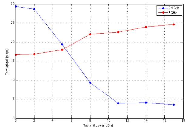
Fig. 14. Throughput of the radio signal crossing through a concrete floor, as a function of the AP transmit power.
