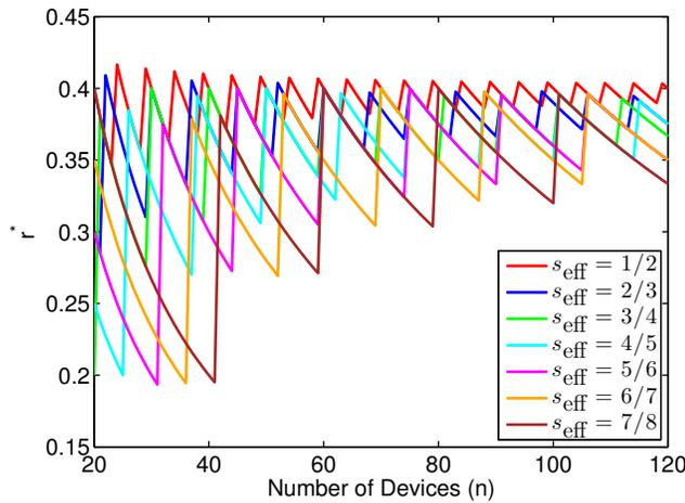
Figure 17.  $r^*$  for  $E(H)$  vs. number of devices for  $s_{\text{eff}} = 1/2, 2/3, 3/4, 4/5, 5/6, 6/7, \text{ and } 7/8$ ;  $\lambda/\mu = 0.001$ .
