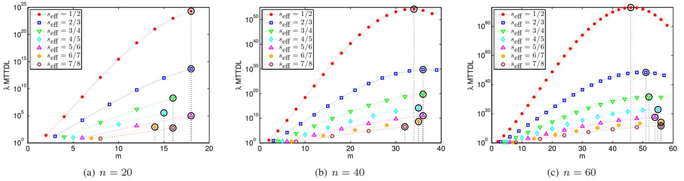
Figure 8. Normalized  $\text{MTTDL}^{\text{declus}}$  vs. codeword length for  $s_{\text{eff}} = 1/2, 2/3, 3/4, 4/5, 5/6, 6/7,$  and  $7/8$ ;  $\lambda/\mu = 0.001$  and deterministic rebuild times.
