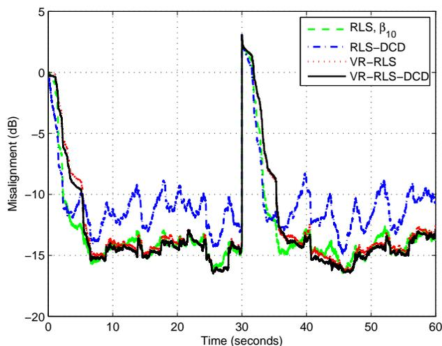
Figure 8. Misalignment of the regularized RLS (using  $\beta_{10}$ ), RLS-DCD, VR-RLS, and VR-RLS-DCD algorithms. The input signal is speech,  $L = 512$ , and ENR = 10 dB. Echo path changes at time 30 seconds.
