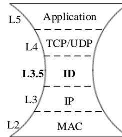
Figure 3. Protocol stack of UPC.
