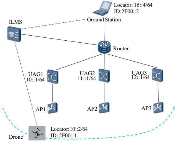
Figure 4. Topology of the drone prototype.
