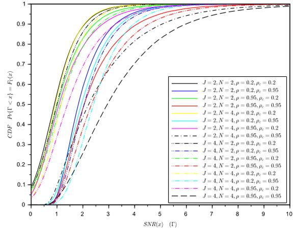
Figure 4. CDF of instantaneous SINR conditional on the estimated SNR being above the threshold  $\hat{\beta} = 2$  with fixed Tx power settings ( $P\gamma/\sigma_v^2 = 1$ ) in the presence of cochannel interference ( $K = 2, \lambda/\gamma = 0.1$ ),  $\kappa = -10$  dB,  $p = 0.7$  and different values of antennas and correlation coefficients.
