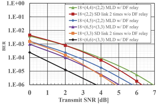
Figure 10. BER characteristics of  $18 \times (4,4) \times (2,2)$  or  $(4,5) \times (2,2)$  and  $18 \times (6,5)$  or  $(6,6) \times (3,3)$  model (Transmission rate to user 1 is 6 (bps/Hz) and 64QAM, 16QAM or QPSK is optimally selected to minimize the BER. Transmission rate to user 2 is 4 (bps/Hz) and 16QAM or QPSK is optimally selected to minimize the BER.)
