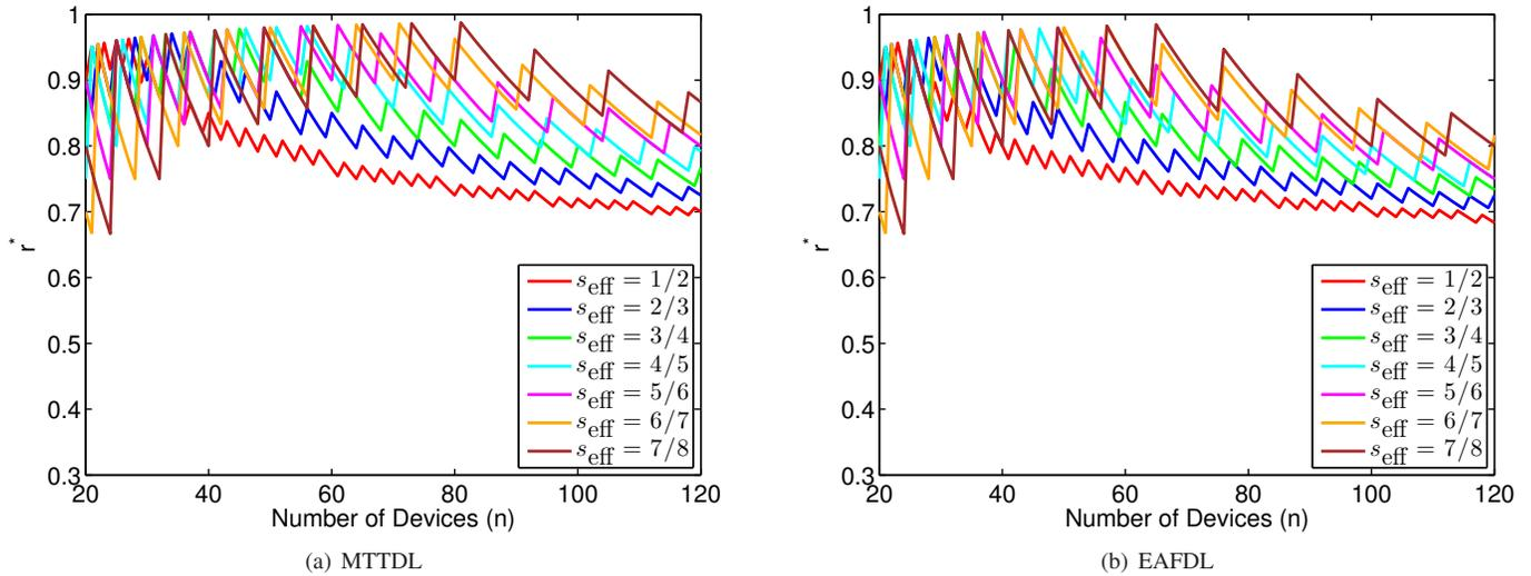
Figure 12.  $r^*$  vs. number of devices for  $s_{\text{eff}} = 1/2, 2/3, 3/4, 4/5, 5/6, 6/7,$  and  $7/8$ ;  $\lambda/\mu = 0.001$  and deterministic rebuild times.
