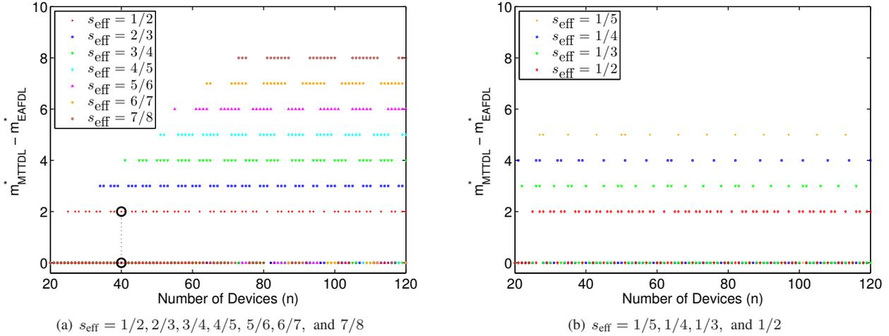
Figure 11. The difference between  $m_{\text{MTTDL}}^*$  and  $m_{\text{EAFDL}}^*$  vs. the number of devices;  $\lambda/\mu = 0.001$  and deterministic rebuild times.
