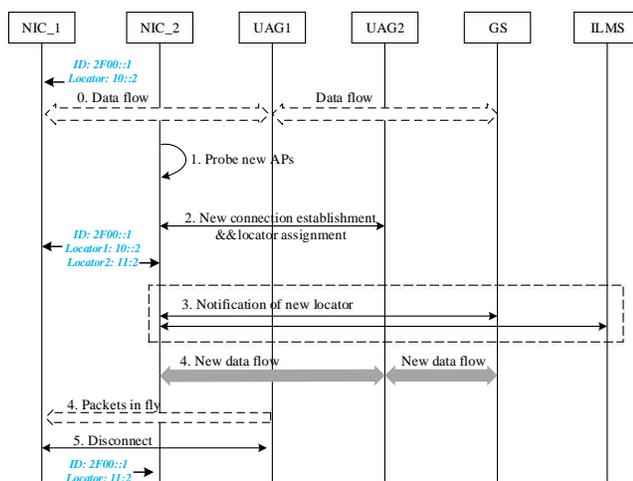
Figure 10. Handover process with two NICs.
