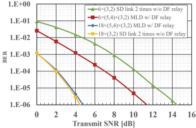
Figure 8. BER characteristics of  $6 \times (5,4) \times (3,2)$  or  $18 \times (5,4) \times (3,2)$  model (Transmission rate to user 1 is 6 (bps/Hz) and 64QAM, 16QAM or QPSK is optimally selected to minimize the BER. Transmission rate to user 2 is 4(bps/Hz) and 16QAM or QPSK is optimally selected to minimize the BER.)
