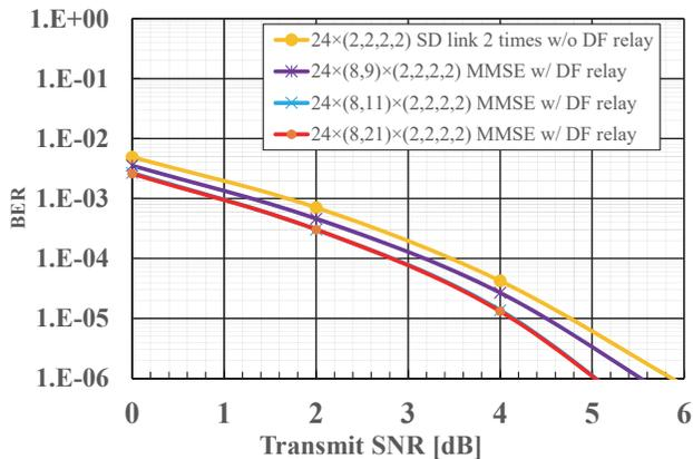
Figure 12. BER characteristics of  $24 \times (8,9)$  or  $(8,11)$  or  $(8,21) \times (2,2,2,2)$  model (Transmission rate to each user is 6 (bps/Hz) and 64QAM, 16QAM or QPSK is optimally selected to minimize the BER.)
