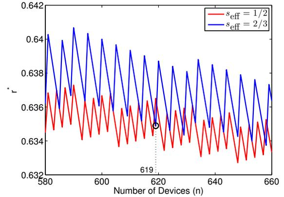
Figure 15.  $r^*$  for MTTDL vs. number of devices for  $s_{\text{eff}} = 1/2, 2/3$ ;  $\lambda/\mu = 0.001$  and deterministic rebuild times.
