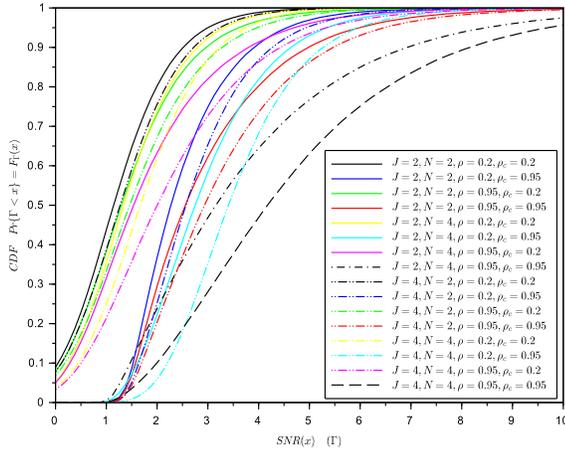
Figure 2. CDF of instantaneous SNR conditional on the estimated SNR being above the threshold  $\hat{\beta} = 2$  with fixed Tx power settings ( $P\gamma/\sigma_v^2 = 5$ ) without interference,  $\kappa = -10$  dB and different values of antennas and correlation coefficients.
