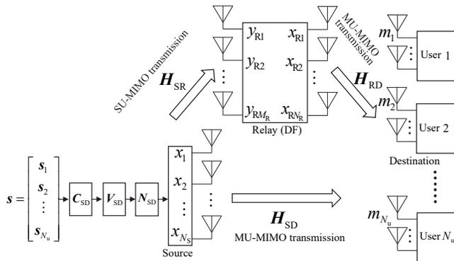
Figure 1. DF relay model in MU-MIMO downlink system
