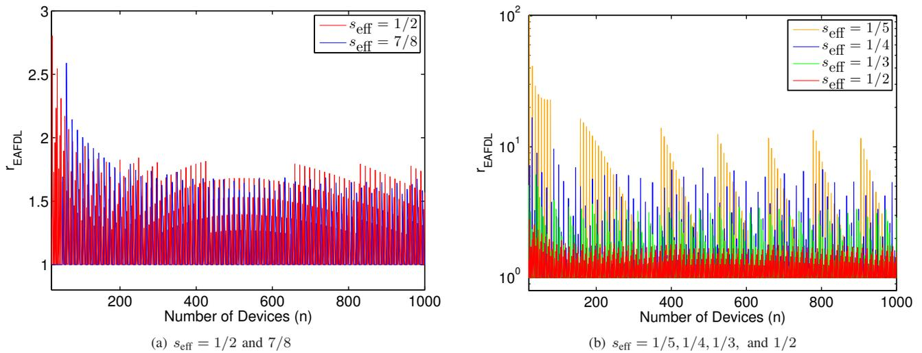
Figure 23. The EAFDL efficiency ratio  $r_{\text{EAFDL}}$  vs. number of devices;  $\lambda/\mu = 0.001$  and exponential rebuild times.
