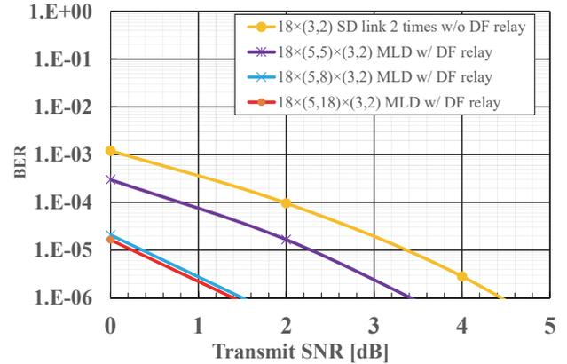
Figure 9. BER characteristics of  $18 \times (5,5)$  or  $(5,8)$  or  $(5,18) \times (3,2)$  model (Transmission rate to user 1 is 6 (bps/Hz) and 64QAM, 16QAM or QPSK is optimally selected to minimize the BER. Transmission rate to user 2 is 4(bps/Hz) and 16QAM or QPSK is optimally selected to minimize the BER.)
