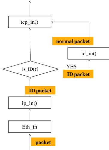
Figure 7. Packet decapsulation process.
