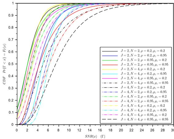
Figure 3. CDF of instantaneous SNR conditional on the estimated SNR being above the threshold  $\hat{\beta} = 2$  with fixed Tx power settings ( $P\gamma/\sigma_v^2 = 5$ ) without interference,  $\kappa = -10$  dB, and different values of antennas and correlation coefficients.
