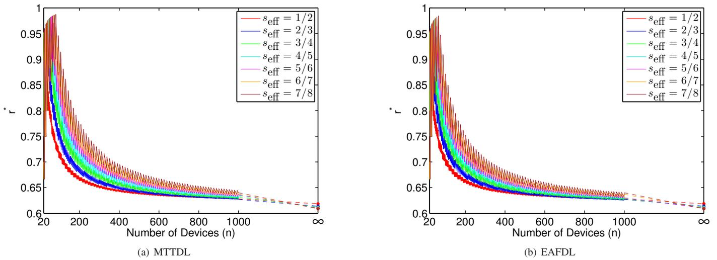
Figure 13.  $r^*$  vs. number of devices  $n \rightarrow \infty$ ,  $s_{\text{eff}} = 1/2, 2/3, 3/4, 4/5, 5/6, 6/7,$  and  $7/8$ ;  $\lambda/\mu = 0.001$  and deterministic rebuild times.
