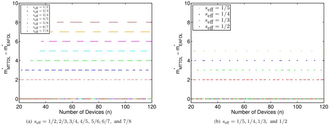
Figure 21. The difference between  $m_{\text{MTTDL}}^*$  and  $m_{\text{EAFDL}}^*$  vs. number of devices;  $\lambda/\mu = 0.001$  and exponential rebuild times.
