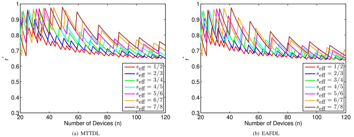
Figure 22.  $r^*$  vs. number of devices for  $s_{\text{eff}} = 1/2, 2/3, 3/4, 4/5, 5/6, 6/7, \text{ and } 7/8$ ;  $\lambda/\mu = 0.001$  and exponential rebuild times.
