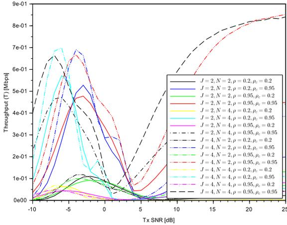
Figure 6. Throughput vs. transmit SNR for the MRC beamforming, scheduling and resource allocation algorithm without interference,  $\kappa = -10$  dB and different vales of antennas and correlation coefficients.
