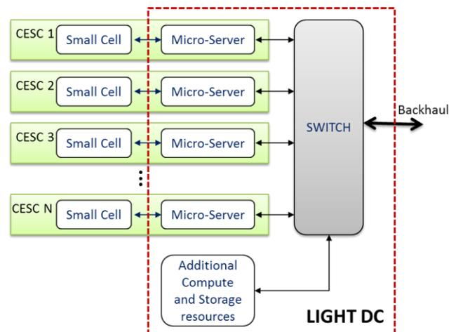
Figure 2. Simplified view of the Light DC Architecture
