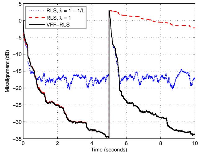
Figure 3. Misalignment of the RLS algorithm (using different constant values of the forgetting factor) and the VFF-RLS algorithm. The input signal is speech,  $L = 128$ , and ENR = 20 dB. Echo path changes at time 5 seconds.
