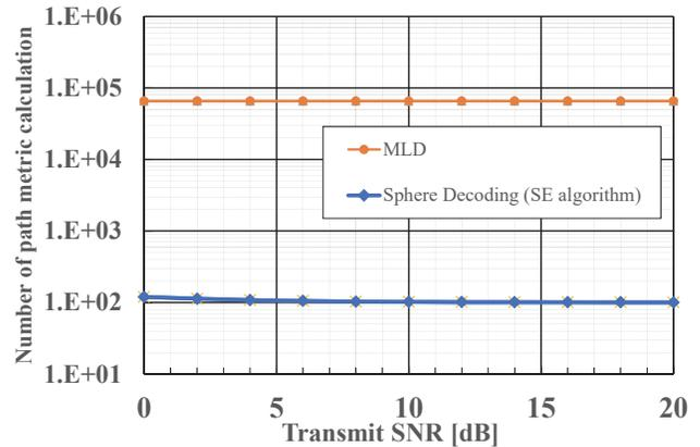
Figure 7. Comparison of number of path metric calculation at DF relay between MLD and Sphere Decoding in  $8 \times (8,8) \times (2,2,2,2)$  model (Transmission rate to each user is 4 (bps/Hz) and 16QAM or QPSK is optimally selected to minimize the BER.)
