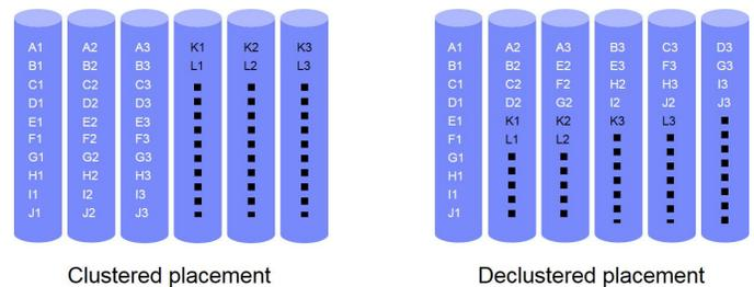
Figure 1. Clustered and declustered placement of codewords of length  $m = 3$  on  $n = 6$  devices. X1, X2, X3 represents a codeword ( $X = A, B, C, \dots, L$ ).
