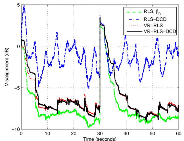
Figure 10. Misalignment of the regularized RLS (using  $\beta_0$ ), RLS-DCD, VR-RLS, and VR-RLS-DCD algorithms. The input signal is speech,  $L = 512$ , and ENR = 0 dB. Echo path changes at time 30 seconds.
