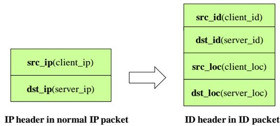
Figure 5. Changes of IP header in ID packet.
