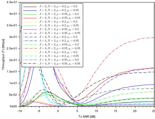
Figure 7. Throughput vs. transmit SNR for the MRC beamforming, scheduling and resource allocation algorithm in the presence of cochannel interference ( $K = 2$ ,  $\lambda/\gamma = 0.1$ ),  $\kappa = -10$  dB,  $p = 0.7$  and different vales of antennas, numbers of terminals and correlation coefficients.
