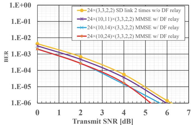
Figure 13. BER characteristics of  $24 \times (10,11)$  or  $(10,14)$  or  $(10,24) \times (3,3,2,2)$  model (Transmission rate to each user is 6 (bps/Hz) and 64QAM, 16QAM or QPSK is optimally selected to minimize the BER.)
