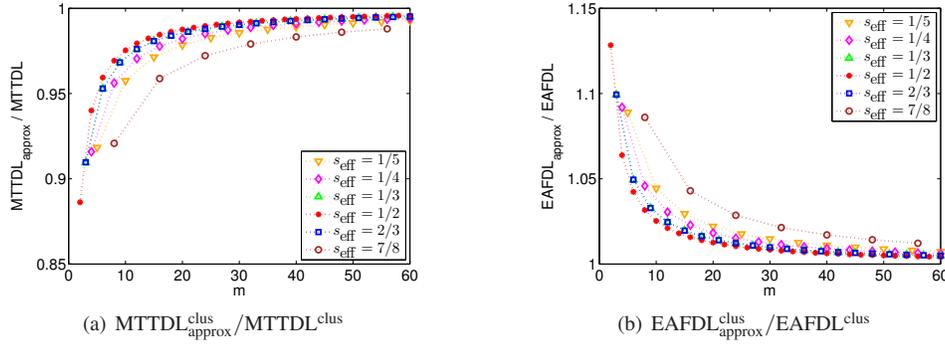
Figure 4. Accuracy of approximations for clustered placement vs. codeword length for  $s_{\text{eff}} = 1/5, 1/4, 1/3, 1/2, 2/3,$  and  $7/8$ .
