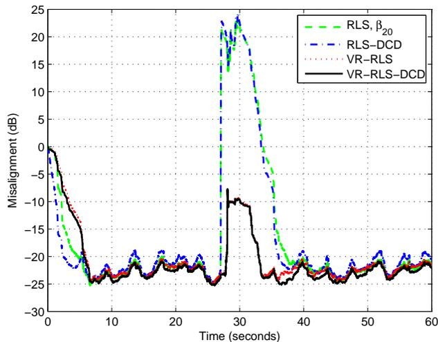
Figure 7. Misalignment of the regularized RLS (using  $\beta_{20}$ ), RLS-DCD, VR-RLS, and VR-RLS-DCD algorithms. The input signal is speech,  $L = 512$ , and ENR = 20 dB. Near-end speech appears between time 27 and 30 seconds (double-talk scenario).
