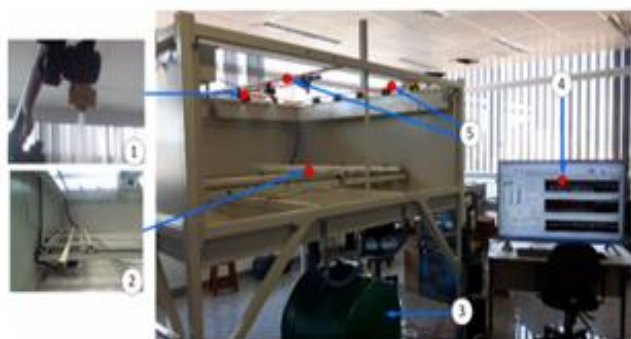
Figure 2. ASDS dedicated to the application of liquid agricultural inputs.
