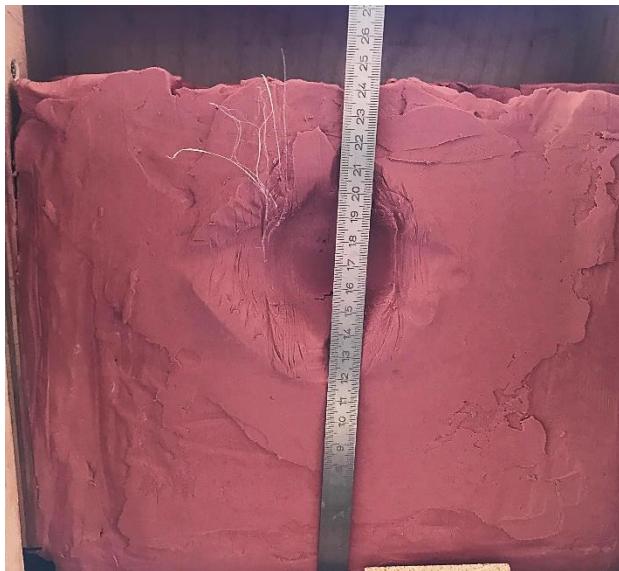
Figure 7. Test number 3 after the shot. Seeable is the volume of the back-face deformation in the clay.
