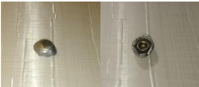
Figure 11. Deformed projectile of test number 12M.
