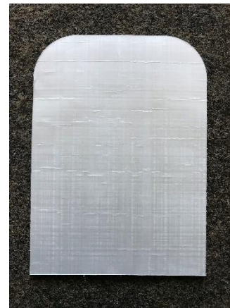
Figure 2. Side body pattern out of Dyneema® HB26. Width of 150 mm and a total height of 205 mm.
