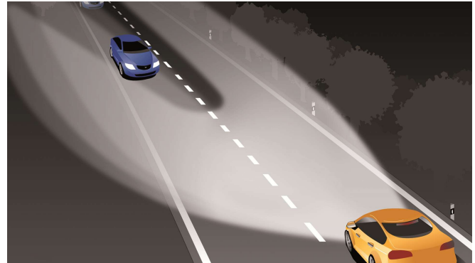
Figure 1. Glare-free highbeam light function cutting off a sharp spatial angle to avoid glaring oncoming traffic. © HELLA
