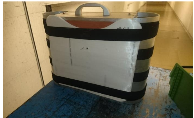
Figure 8. Test number 12M after the first shot. Seeable is the principle test setup, based on VPAM BSW.
