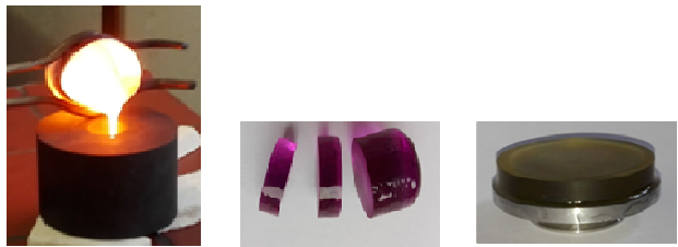
a) Pouring of molten glass in a graphite mold b) Targets of pH glass c) pH glass target fixed on target holder
