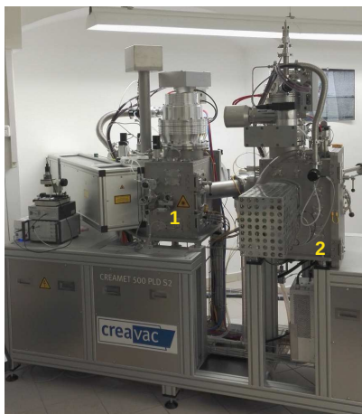
Figure 7. Combined coating system with PLD (1) and sputter (2) chamber
