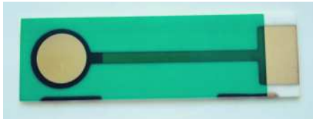
Figure 11: pH thin film electrode
