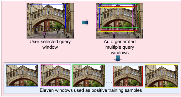
Figure 2: Auto-generation of offset windows to be used as positive training samples during querying. The window dimensions and offsets shown are only representative.
