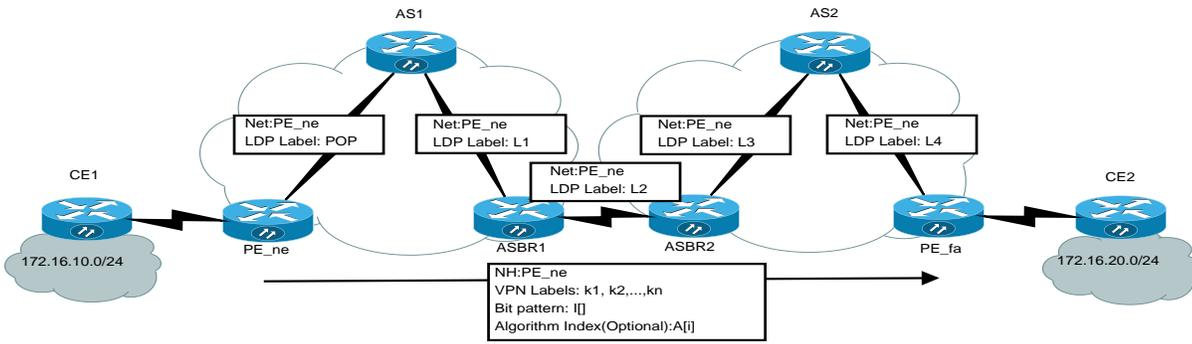
Fig. 1: Control-plane exchanges for model “C” [10]
