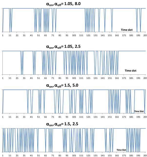
Figure 14. Bursty parameter and traffic patterns
