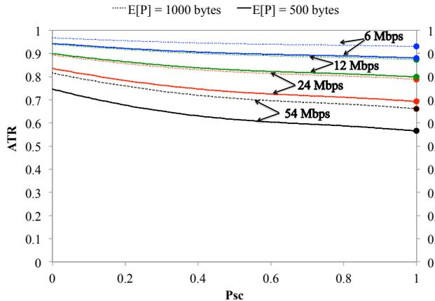
Figure 5. ATR characteristics with respect to the success probability,  $P_{sc}$ . Note that the solid (dashed) lines correspond to 500 bytes (1000 bytes) of data size. The figure clearly shows that ATR is maximized when  $P_{sc}$  is minimized. The optimal value of ATR (that maximizes  $P_{sc}$ ) is smaller than the maximum value of ATR. The figure also shows that the larger the data rate, the smaller is the ATR and the larger the data size, the larger is the ATR.
