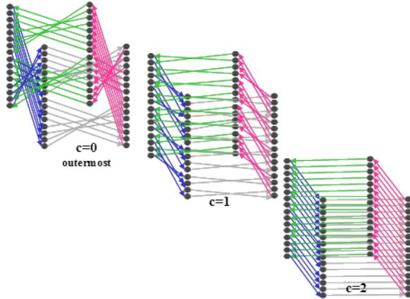
Figure 21. Routing patterns at each of the three cylinders in a 4-ary decoding Data Vortex network.  $A=4, H=16, C = \log_4 H + 1 = 3$
