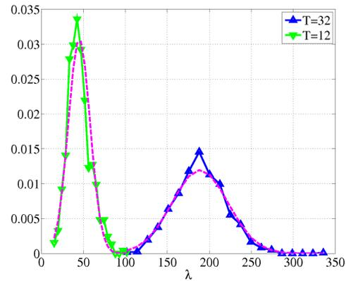
Fig. 5. Probability density function of the smallest signal eigenvalue of a matrix  $\hat{\mathbf{R}}^\dagger$  in the signal-bearing case with  $K = 4$ , i.e.  $\lambda_5$ , with  $m = 61440$ , a noise variance of  $\sigma^2 = 0.1$ , and different values for  $T$ . The solid curves with markers are the simulation results and the dotted curves are the Gaussian distribution.
