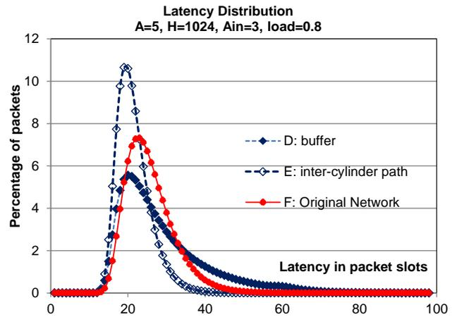
Figure 13. Latency distribution for D, E and F in Fig.11
