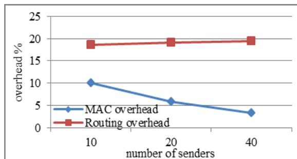
Figure 8C. Control Overhead vs Senders
