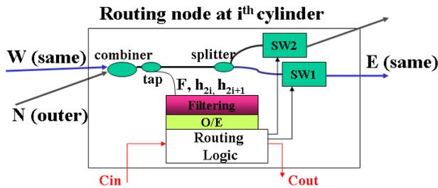
Figure 22. Routing node of 4-ary network that requires two header bits detection
