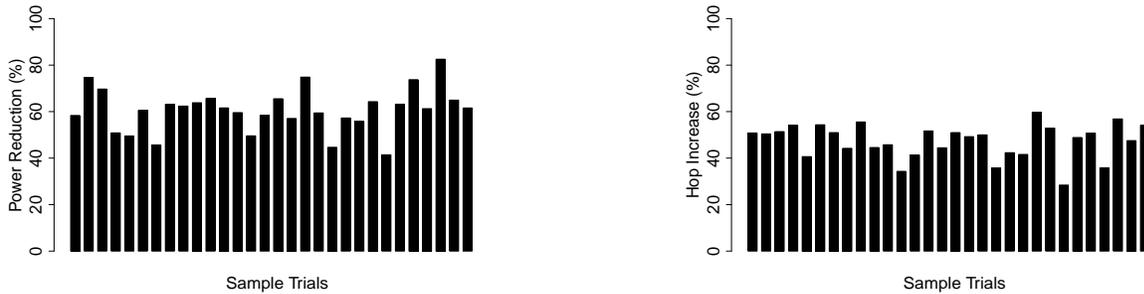
Fig. 6. Power reduction and hop increase for *exponential distribution* of power values with 70% connectivity.
