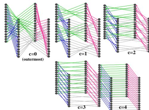
Figure 1. Data Vortex network with Angle=4, Height=16 and Cylinder=5 and its layout of routing node at different cylinders
