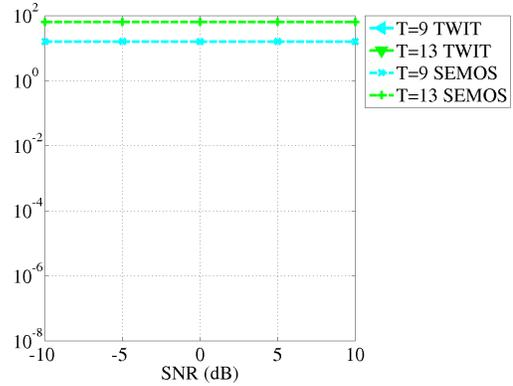
Fig. 11. MSE of two estimation techniques (the SEMOS estimator and the TWIT criterion) for  $K = 4$ , a variable number of snapshots  $T$ ,  $5 \leq T \leq 15$ , and different SNR values, in the presence of a colored noise.
