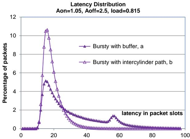
Figure 17. Latency distribution performance comparison
