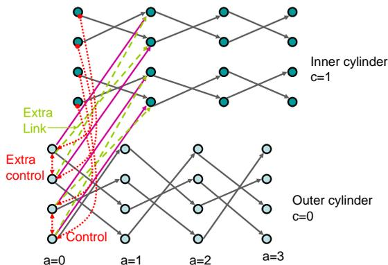
Figure 6. Extra inter cylinder path in Data Vortex network with required extra control
