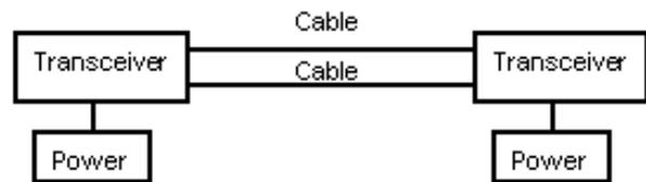
Figure 7. Partially Protected Link
