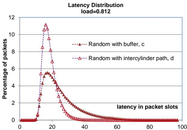
Figure 18. Latency distribution performance comparison
