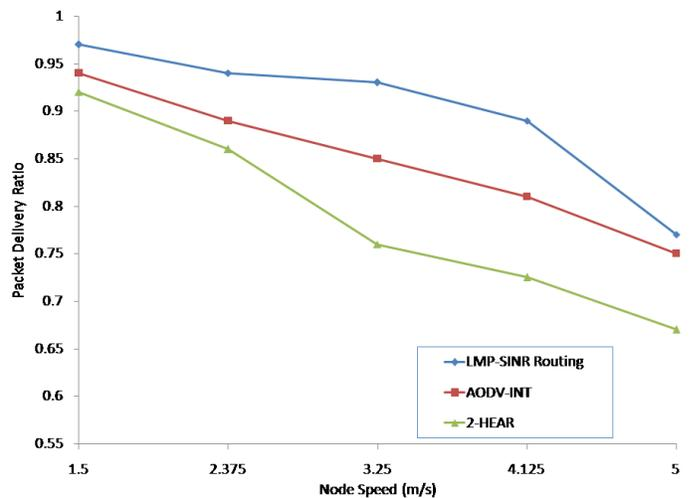
Fig. 7. Packet delivery ratio versus varying node speeds for  $T = 10\text{ms}$
