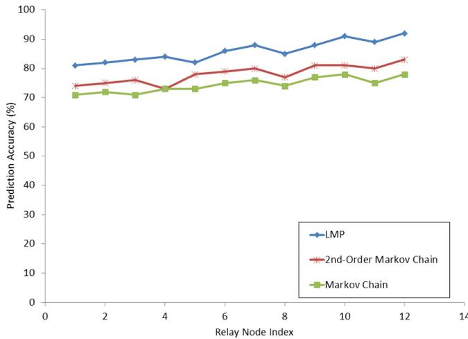
Fig. 5. Comparison of prediction accuracy for the proposed LMP algorithm, generic Markov chain and second-order Markov chain for User Node 1 in networks with 120 users, 14 relay nodes and 1 base station
