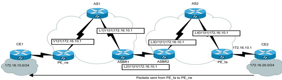
Fig. 3: Data-plane flow for model “C” [10]
