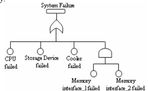
Figure 13. Fault tree model of System Failure
