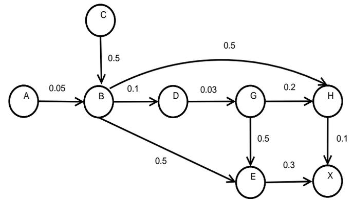
Fig. 2. Strands combined to get the Internet topology. The PWR metric is mapped to the ingress link of the ASBR. CSPF algorithm is run on this topology to detect the low-power path by the PCE.
