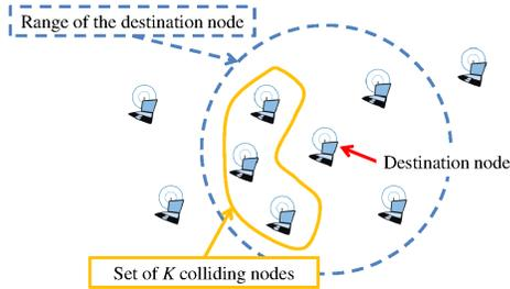
Fig. 1. Collision Scenario with  $K = 3$  colliding nodes.
