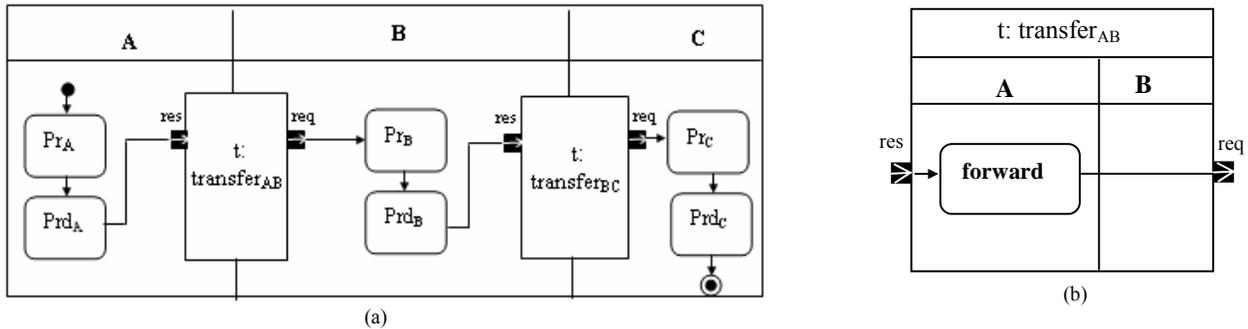
Figure 3. (a) Detail behavior of the event of the collaboration using activity (b) internal behavior of the collaboration
