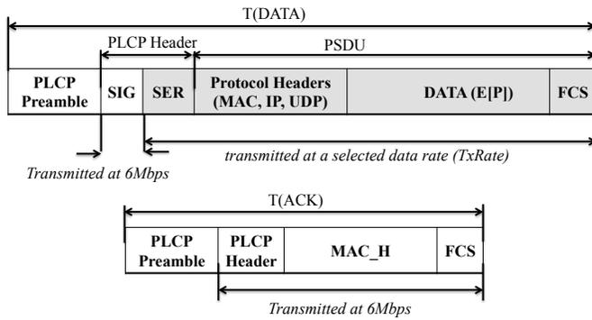
Figure 3.  $T'$  the sum of the times required for transmissions of a data frame and the corresponding acknowledgment frame. PLCP SIGNAL field duration and ACK frame are generally coded with 1/2 BPSK (i.e., 6 Mbps rate) in the IEEE 802.11a systems. The shaded area of the data frame is transmitted at a rate ( $TxRate$ ) selected by the MAC rate adaptation mechanism.
