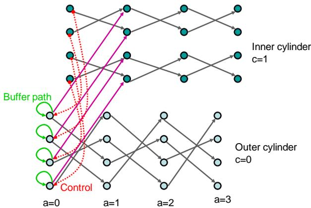
Figure 4. Data Vortex network with buffers within node shown at  $a=0$ .
