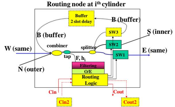
Figure 5. Routing node with buffer implementation: a 2-slot delay for buffer path is necessary to setup the control signal on time and additional controls  $C_{out2}$  are used to inform the state of buffer
