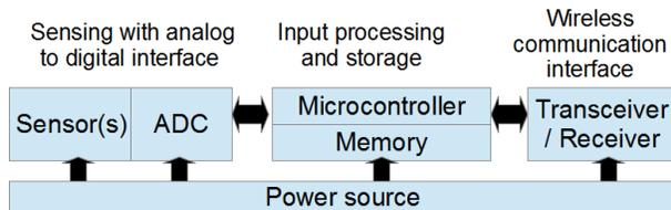
Figure 1. Block diagram of wireless sensor module
