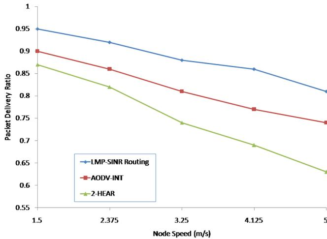
Fig. 8. Packet delivery ratio versus varying node speeds for  $T = 1ms$
