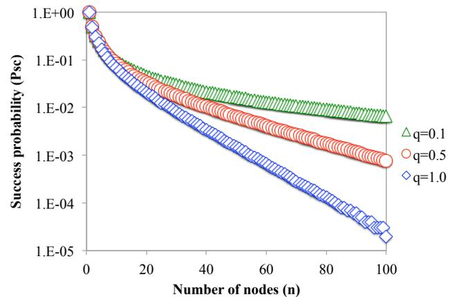
Figure 2. Success probability as a function of the number of contending nodes. The figure shows that  $P_{sc}$  sharply decreases with the increase of the number of nodes. The smaller the probability of having a pending frame ( $q$ ), the larger is the  $P_{sc}$ .
