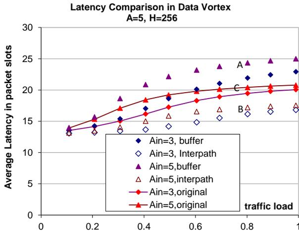
Figure 8. Latency comparison under various traffic load and redundant conditions
