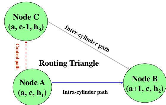
Figure 3. Control Signal in Routing Triangle
