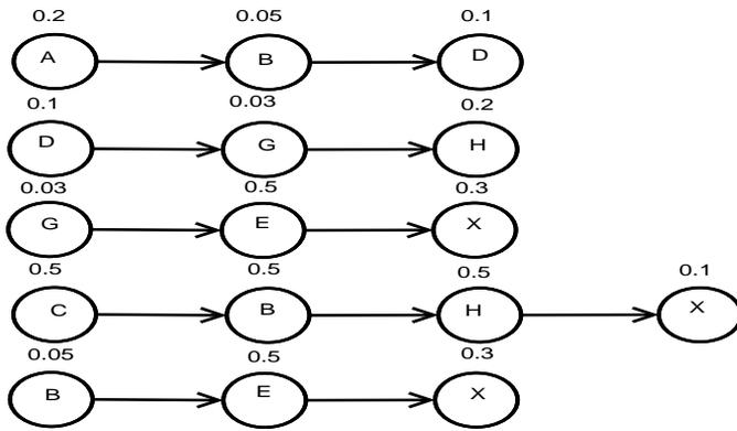
Fig. 1. Strands obtained from BGP updates, vertices  $A, B, C, D$  and  $G$  are the head-end AS;  $D, H$  and  $X$  are the tail-end AS. The vertex weights represent the PWR metric of an AS, and the link direction shows the next AS hop. ASBRs present the topology to the PCE.
