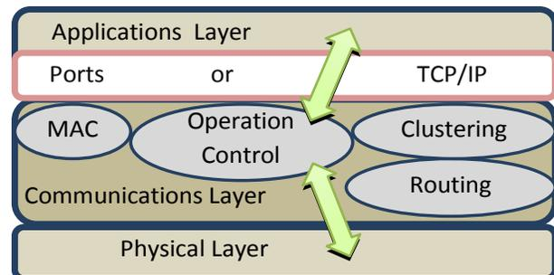
Figure 1 The Integration Architecture
