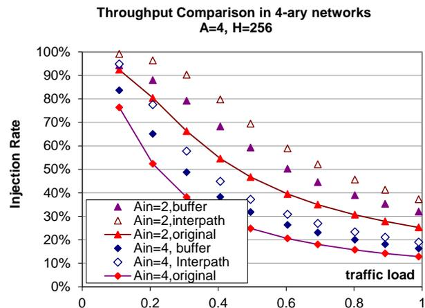
Figure 24. Throughput performance comparison
