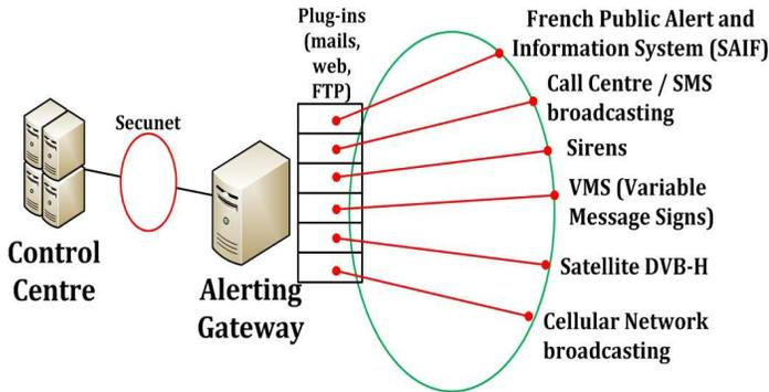
Figure 10. Demonstration of the public Alerting System
