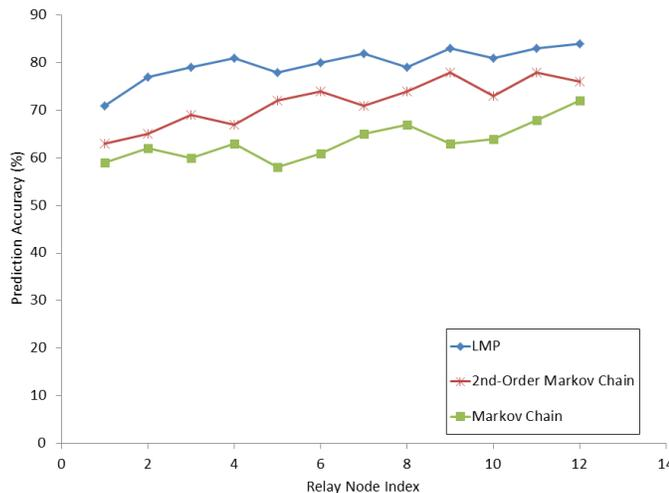
Fig. 6. Comparison of prediction accuracy for the proposed LMP algorithm, generic Markov chain and second-order Markov chain for User Node 2 in networks with 120 users, 14 relay nodes and 1 base station
