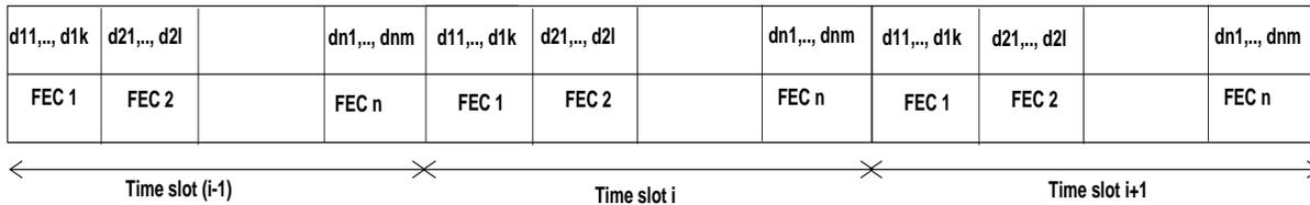
Fig. 5: Total distinct valid keys for a particular time slot  $i$ , various FECs  $j$  in a TicToc based protection against spoofing attacks. In case the keys are too large then a random seed which can generate the keys  $d_{ijk}$  can be exchanged. In this case,  $PE_{fa}$  and  $PE_{ne}$  must know the random number generation algorithm a-priori.
