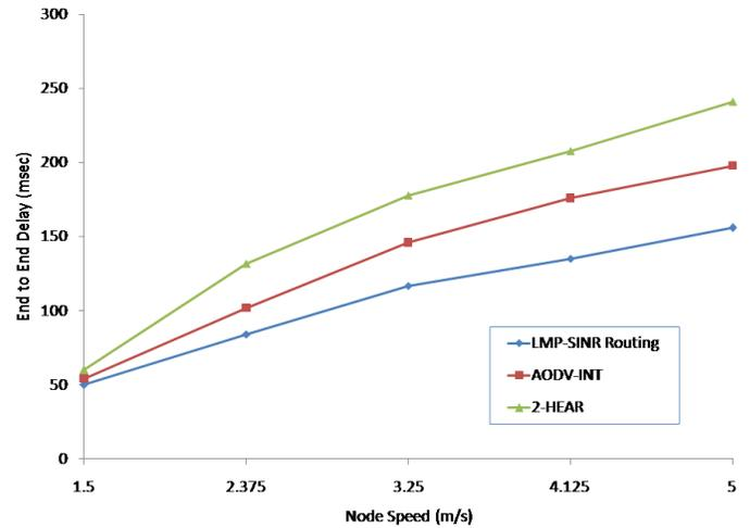
Fig. 10. End-to-end delay for  $T = 1ms$  and varying node speed
