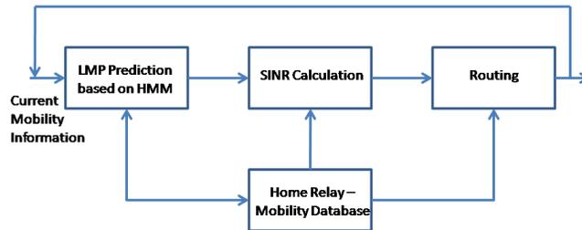
Fig. 2. Block diagram that illustrates the interaction between the LMP algorithm and the interference aware routing algorithm. The home relay runs the prediction algorithm and the SINR calculation for the routing procedure
