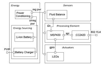
Figure 10. Fluid balance sensor node internal block diagram.
