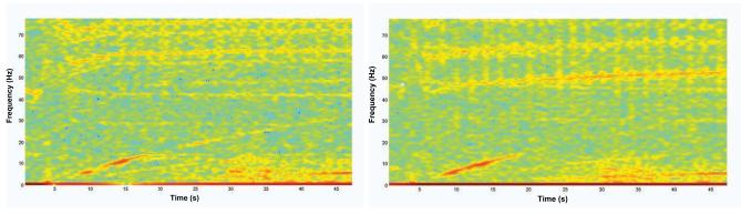
(a) Spectrum carriage 1, train 1, x-axis(b) Spectrum carriage 2, train 1, x-axisFigure 7. Frequency spectrum x-axis of two carriages in the same train
