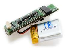
Figure 11. ASE-BAN node (fluid balance sensor side).
