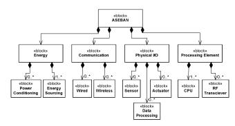
Figure 5. ASE-BAN node hardware block diagram.
