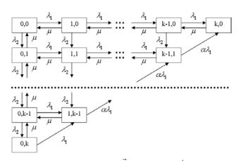
Figure 10. The state graph of  $\vec{M}_2 / M / 1 / k / f_2^1$  type system
