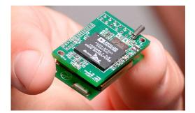
Figure 20. The ASE-BAN ECG sensor module with DSP. The size is 13 mm x 18 mm x 30 mm. The weight is 6 g.
