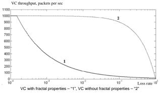
Figure 8. Dependence of TCP throughput on packet loss probability for TCP connections
