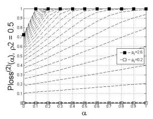
Figure 11. Loss probability of non-priority packets with 0.1 step for  $0.2 \le \rho_0 \le 2.6$ , buffer size 31 and weak non-priority stream
