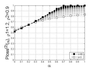
Figure 14. Loss probability of non-priority packets with buffer size K=3- $\frac{80}{80}$
