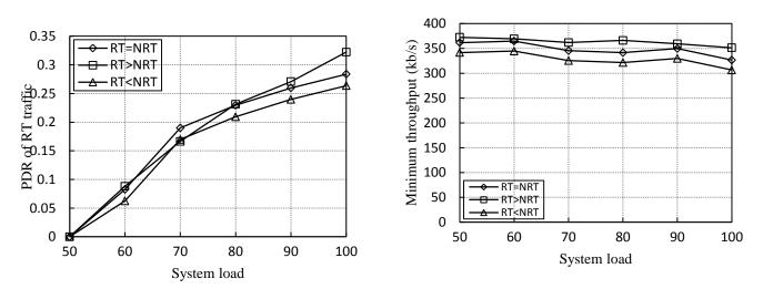
Figure 11. PDR of RT traffic and minimum throughput of NRT traffic.
