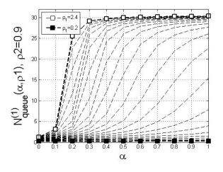
Figure 16. Average priority queue length with medium intensity of second stream with buffer size 31
