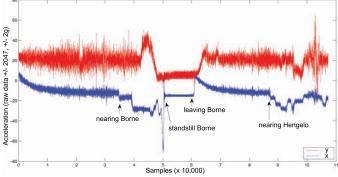
Figure 6. Accelerometer x- and y-axis
