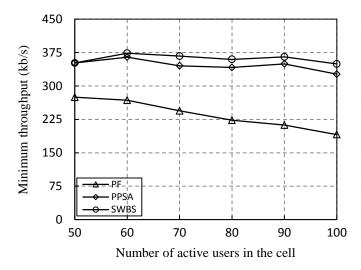
Figure 7. Minimum throughput of streaming video traffic.
