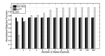
Figure 8. Objective function value normalized to the optimal solution for a varying number of states explored for the one-shot, greedy, and SA algorithms for an ambient conditions monitoring application where  $\omega_l =$ 0.4,  $\omega_t = 0.5$ ,  $\omega_r = 0.1$ , |S| = 31, 104.
