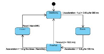
Figure 21. The four states of the fall detection algorithm.
