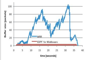
Figure 15. Buffer Size of Receiver Middleware
