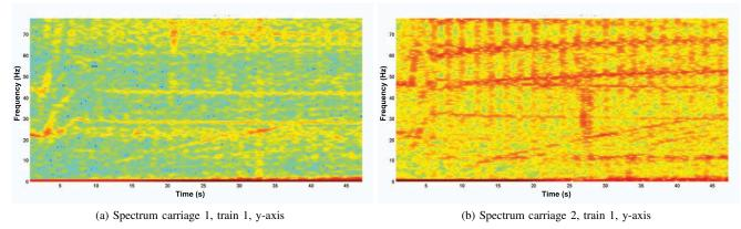
Figure 8. Frequency spectrum y-axis of two carriages in the same train
