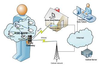
Figure 1. A wireless body area network system.
