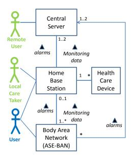
Figure 3. System domain model including ASE-BAN.
