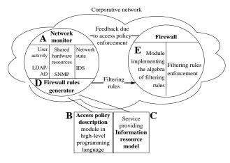
Figure 4. Security monitor architecture
