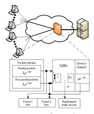
Figure 9. Priority queueing schema  $M_2/M/1/k/f_2^1$  of telematics network devide
