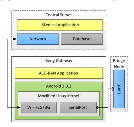
Figure 14. Central server and body gateway software components.
