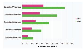
Figure 12. Execution times on a muNode with MSP430 microcontroller
