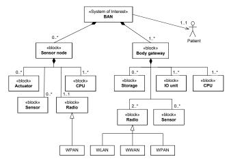
Figure 4. Block definition diagram describing the ASE-BAN architecture.
