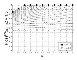
Figure 12. Loss probability of non-priority packets with 0.1 step for  $0.2 \le \rho_{\rm s} \le 2.6$ , buffer size 31 and more ntensive non-priority stream
