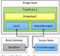
Figure 15. Bridge node software components
