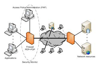
Figure 1. Firewall as a central component of access policy enforcement
