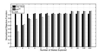
Figure 7. Objective function value normalized to the optimal solution for a varying number of states explored for the one-shot, greedy, and SA algorithms for an ambient conditions monitoring application where  $\omega_l =$ 0.4,  $\omega_t = 0.5$ ,  $\omega_r = 0.1$ , |S| = 729.
