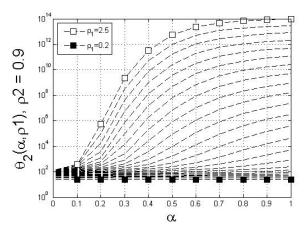
Figure 20. The time that non-priority packet spend in queueing built in logarithmic y scale
