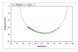
Figure 18. Cole plot of a network with two series-connected resistors of 75  $\Omega$  each and one capacitor of 220 nF in parallel to one of the resistors with the approximating circle. The frequency range was from 5 kHz (rightmost data point) up to 25 kHz using 250 Hz of step size.
