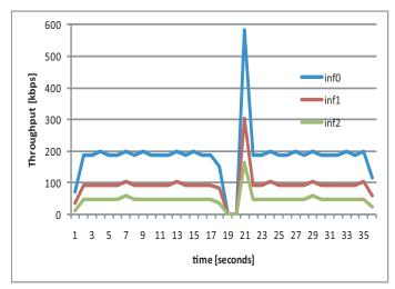
Figure 17. Throughput of Bandwidth Aggregation on Middleware with Packet Loss
