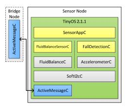
Figure 16. Sensor node software components.
