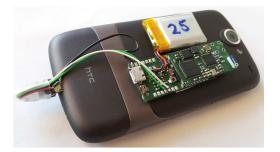
Figure 24. Body gateway with bridge node.
