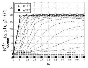
Figure 15. Average priority queue length with low intensity of second stream with buffer size 31
