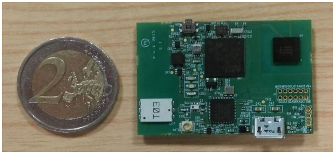
Fig. 1. Tyndall Wireless Inertial Measurement Unit (WIMU).
