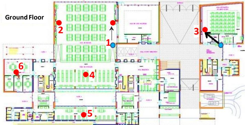
Figure 20. Relocation of APs on the ground floor
