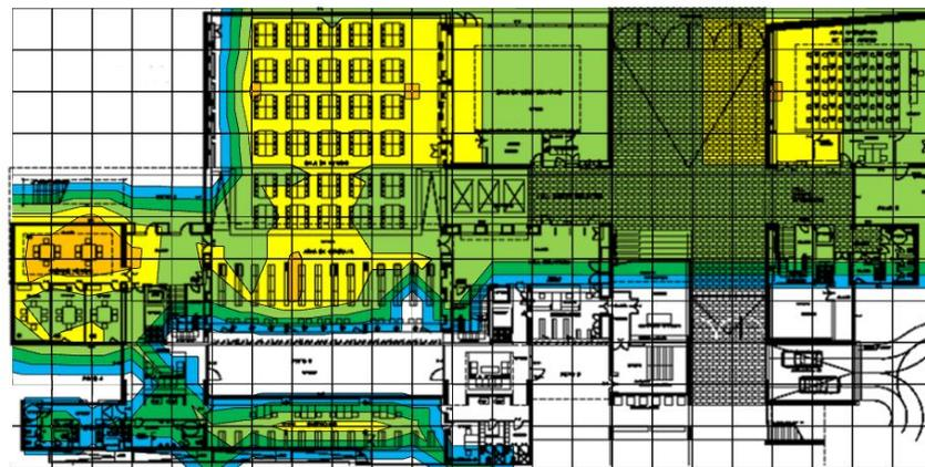
Figure 21. Estimated signal strength on the ground floor for the proposed AP relocation.
